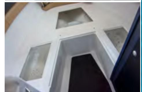
The **pantry block** made of an easy-care and rounded GRP molding contains a large sink with pre-installed water drain, side ventilation windows and a skylight.
